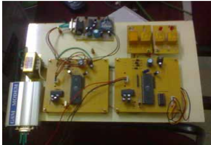
Main control unit and GSM module
